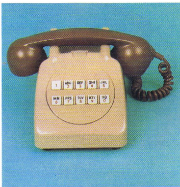
(g) Telephone No. 724 (experimental press-button configuration—2 × 5)—1966
